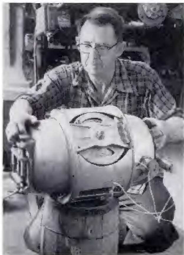
While telephone-line crew waits, he drops other work to rush repairs on automatic cable-hanging machine
